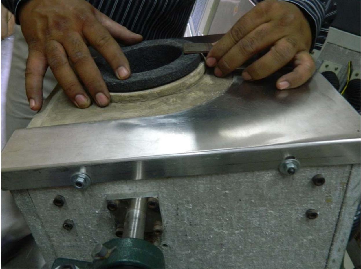
**Securing Crucible by sliding support**
